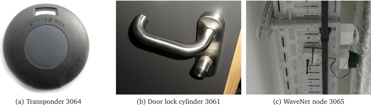
Figure 5.1: Components of the SimonsVoss 3060 digital locking system
